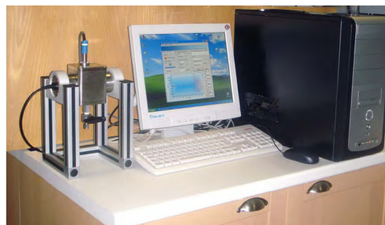
Figure 3 Picture of the prototype C-V device
