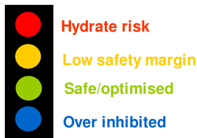
Figure 1 Hydrate safety margin determined by the developed hydrate monitoring technique could be used as traffic lights to help the operators have a better control of hydrate inhibition.
